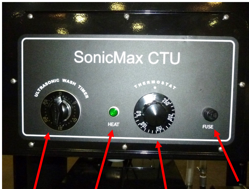
Heater ON pilot light Ultrasonic Timer Thermostat Heater Circuit Fuse
