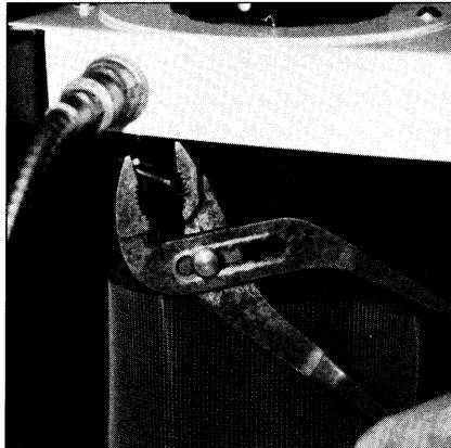
5. Use pliers to loosen wire clamp and slide up to secure hose.
