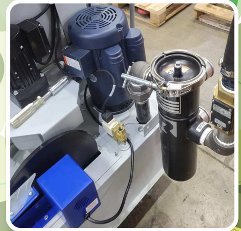
Filter Upgrade & Skimmer
