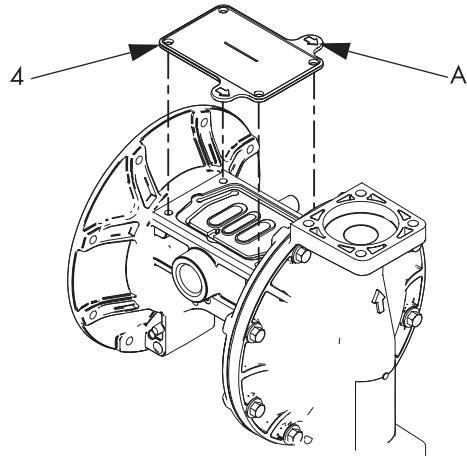
2. To ensure proper seating and extend diaphragm life, attach the second fluid cover with air pressure of the pump.
