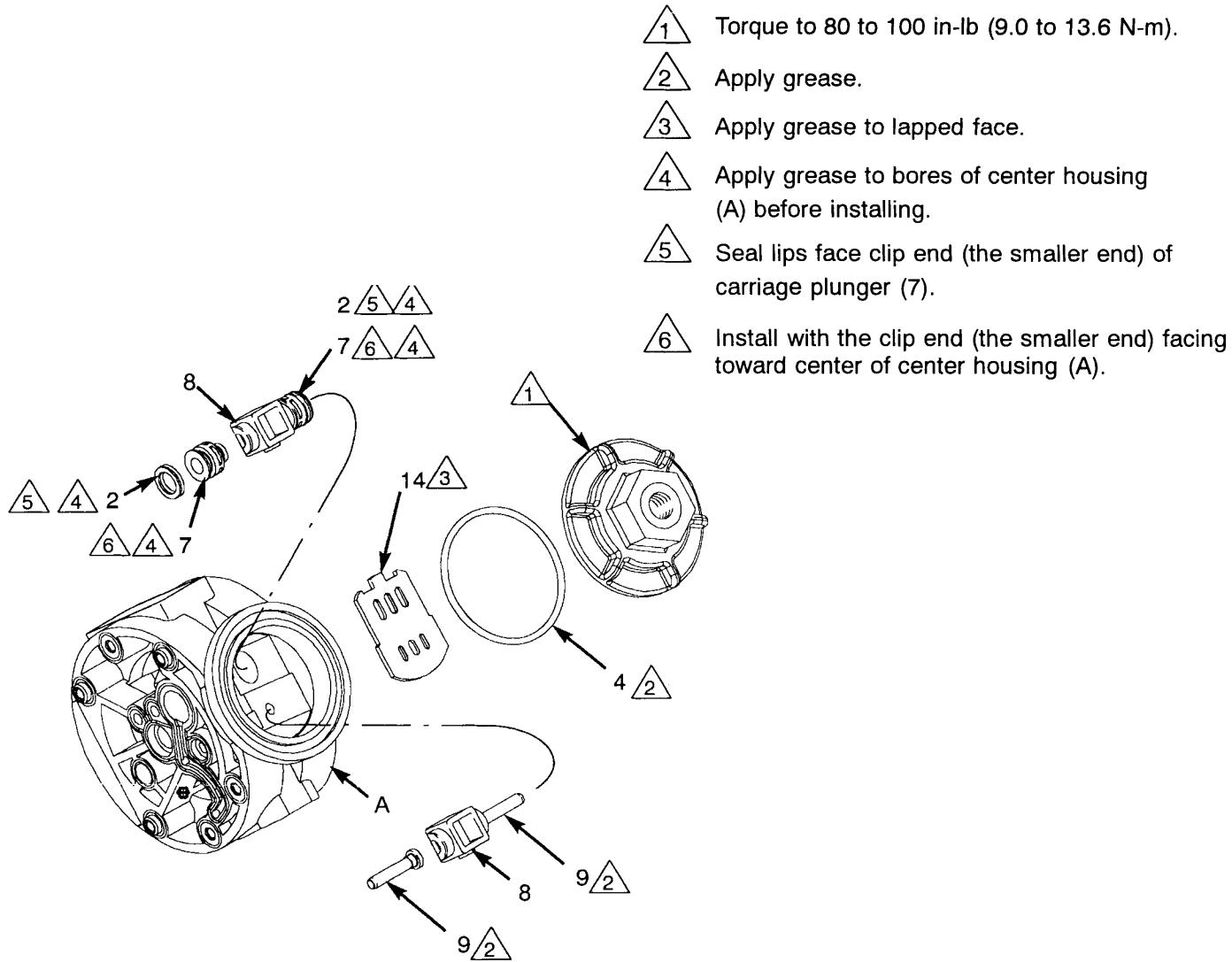
**NOTE:** Center housing (A) is shown separated from the air covers, but it is not necessary to remove the air covers for this service. Leave the center housing and air covers assembled for this service.
